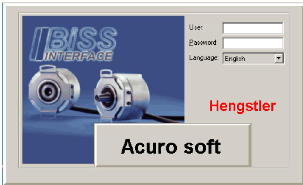
A "blank" entry (using the return key) is a permissible user entry. A password is not required. The "blank" user has exclusive read access on the encoder - this will be sufficient for checking the encoder functions.
