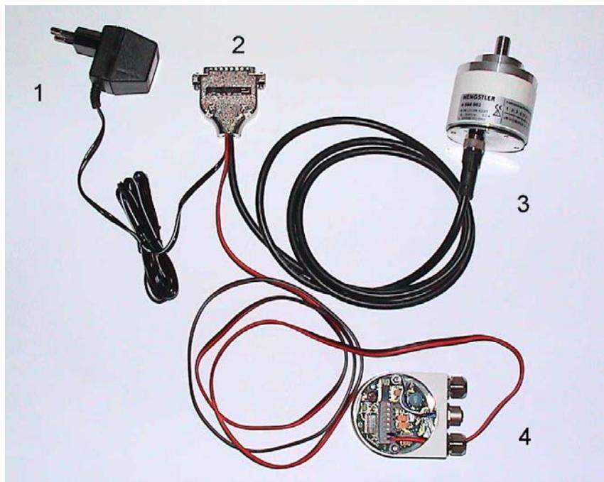
Open the encoder by removing the screws on the upper side. Pull the bus cover off the encoder base. Connect the M12 plug (3) on the upper side of the encoder base.
