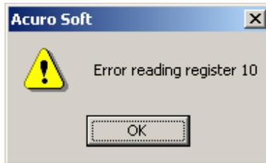
Possible cause: Encoder connection error or incorrect installation of encoder; no voltage supply (please check the status LED on the encoder)
