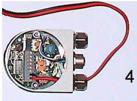
Re-assemble the encoder, tighten the screws and connect the "tico" indicator **(5)** to the center terminal of the bus cover. (Note that this connection will not be possible for all encoder/bus cover types).
