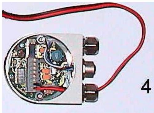
Connect the ACURO industry encoder base to the parallel (PRINTER) interfaces of your PC by means of the 25-pole Sub-D connector **(2)** and plug the power supply **(1)** into a 220V socket. The power supply is used to supply power to the encoder and the electronics included in the Sub-D connector.
