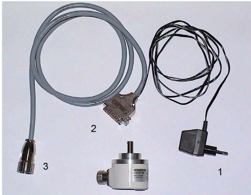
Connect the adapter cable to the ACURO industry encoder to by means of the 12-pin round plug **(3)** and to the parallel interface (PRINTER) of your PC by means of the 25-pin SUB-D plug **(2)**.
