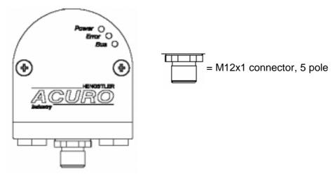
$\Rightarrow$  Connect the encoder to the bus trunk via a drop line
