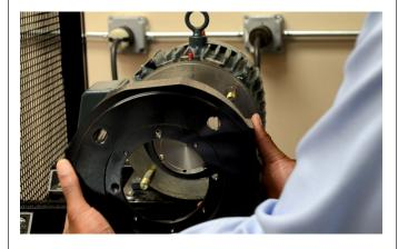
2. Remove the cover if installed by removing (2) 1/2"-13 UNC Acorn Nuts
