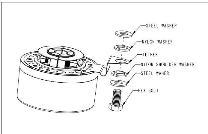
Slide the flat nylon washer on the side away from the bend and the flanged nylon washer on the side of the bend and press them together until they are fully seated in the tether hole. One steel washer is to be used on each side of the nylon washer.
