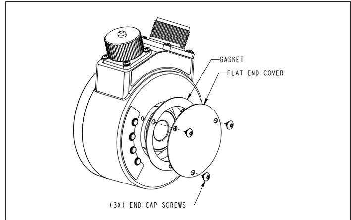
The encoder ships with an endcap to cover the back end of the encoder body and, although optional, it is recommended for additional environmental protection. To install, remove the factory installed three screws at the back of the encoder, properly discard the removed back plate and the three screws. Unpack the endcap, gasket and the three screws from the factory supplied kit. Align the three holes and fasten the gasket and end cap to the encoder body as shown.
