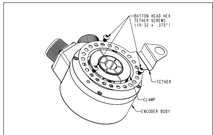
Rotate the tether to the required orientation and tighten the tether arm to the encoder body using the three screws provided. The hollowshaft series encoder tethers can be rotated in 15 degree increments so that connector or cable exit can be conveniently located.
