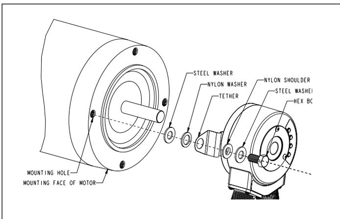
Rotate the tether arm until it is at the correct orientation and is aligned with the mounting holes on the the motor or equipment. Install one steel washer on both sides of the nylon washer. Refer figure above. Fasten the tether arm to the motor or machine housing using the supplied 3/8" bolt (4.5" C-face applications) or 1/2" bolt (8.5" C-face applications). Ensure that there is no stress or flexing of the tether arm when secured.
