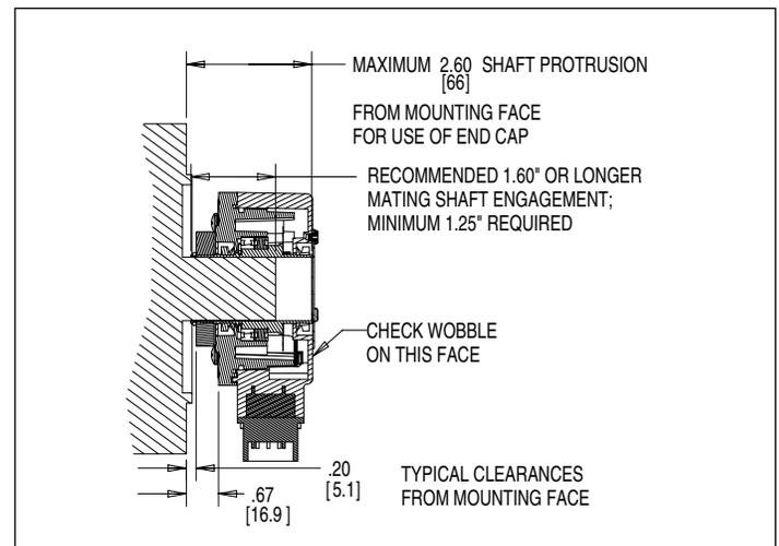
Follow the 3 step installation check to ensure a good installation thus far. Refer to figure above for key reference dimensions
