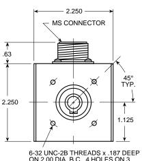
6-32 UNC-2B THREADS x .187 DEEP ON 2.00 DIA. B.C., 4 HOLES ON 3 FACES (FRONT, REAR & BOTTOM). FOR MODELS 22M ONLY: M3 x 0.5-6H
