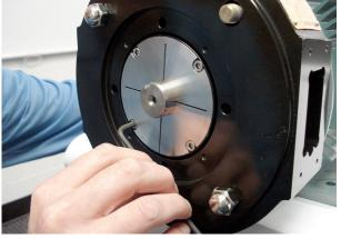
6.1 Tighten (4) M5 X .08 screws in a star pattern (nominal 35 in-lbs) to secure the wheel in the correct position.
