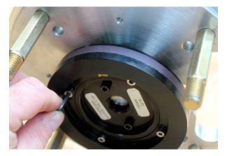
Insert the 4 - M4x 0.7mm Socket Head Cap Screws into the through holes. Tighten to ~ 20 inch-pounds. "Low Strength" Thread-locker is suggested.
