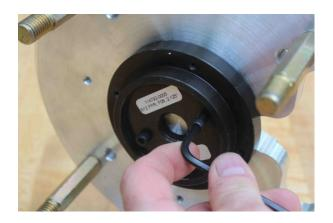
Orient the Shaft adapter to end of the motor. The fit should be snug, but smooth. The labels should be visible and away from the motor.
