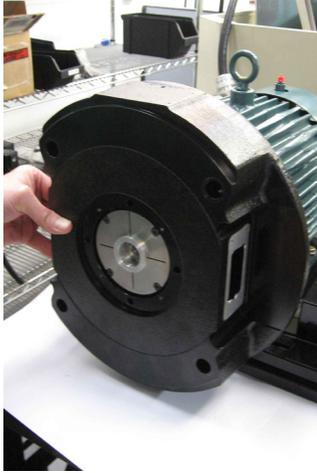
2.4 Tighten 5/8" x11 UNC Hex head cap screws (nominal 125 ft-lbs) into the housing, check to insure the heads seat tight to the Housing.
