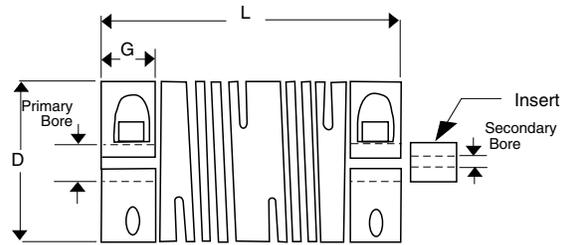
integral 360° clamps which firmly grip the encoder shaft and the input shaft while remaining slip-free to the rated torque of the coupling. NOTE: Shafts may extend beyond the clamp-grip area (G) to the flexure area but they must not butt.
