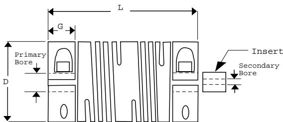
Attachment of a flexible coupling at both ends is via integral 360° clamps which firmly grip the encoder shaft and the input shaft while remaining slip-free to the rated torque of the coupling. NOTE: Shafts may extend beyond the clamp-grip area (G) to the flexure area but they must not butt.
