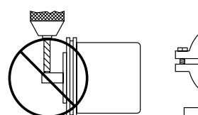
Do not tool the encoder or its shaft.
