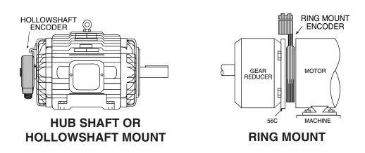
A hub shaft or hollowshaft encoder should be mounted so that its shaft receptacle is in as close as possible alignment with the axis of the driving machine or motor shaft. Clamp or set screws should then be tightened to secure the encoder. NOTE: Do not defeat or restrict the flexure. This causes failure of the encoder or driving shaft bearings.
