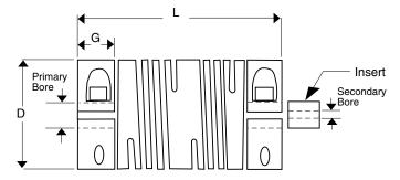
Attachment of a flexible coupling at both ends is via integral 360° clamps which firmly grip the encoder shaft and the input shaft while remaining slip-free to the rated torque of the coupling. NOTE: Shafts may extend beyond the clamp-grip area (G) to the flexture area but they must not butt.
